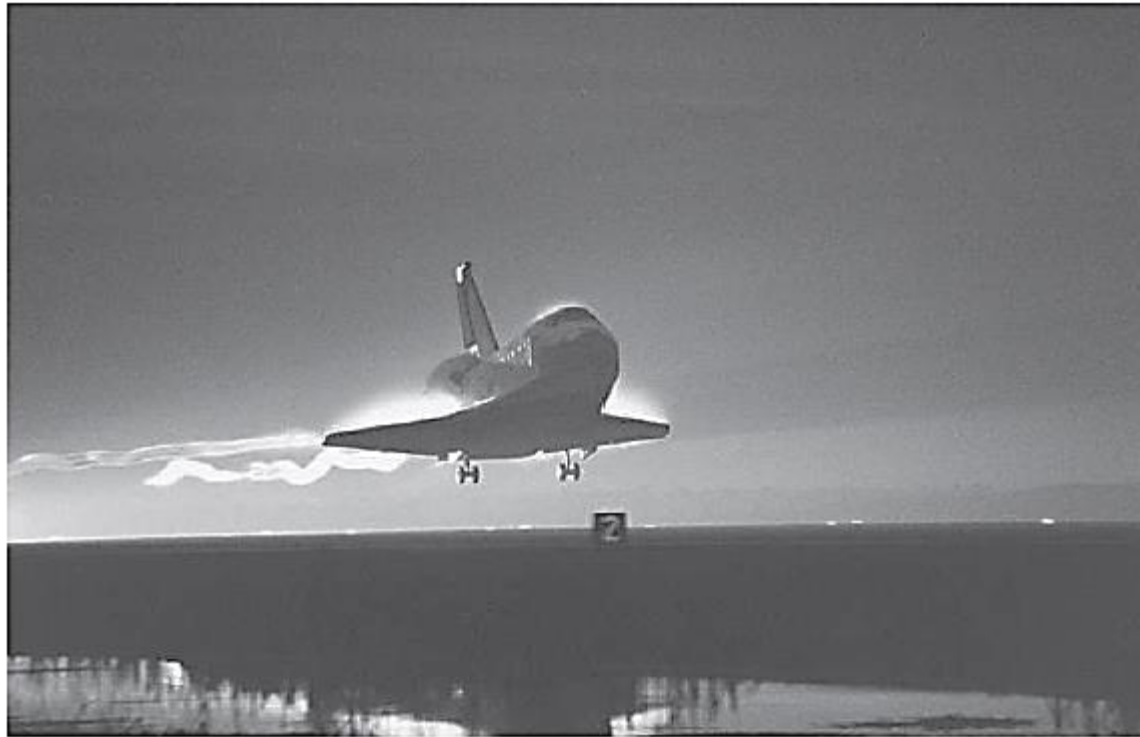
Figure 7.3 Condensation marks the wing-tip vortices of the Space Shuttle Orbiter Columbia (photo courtesy NASA).
