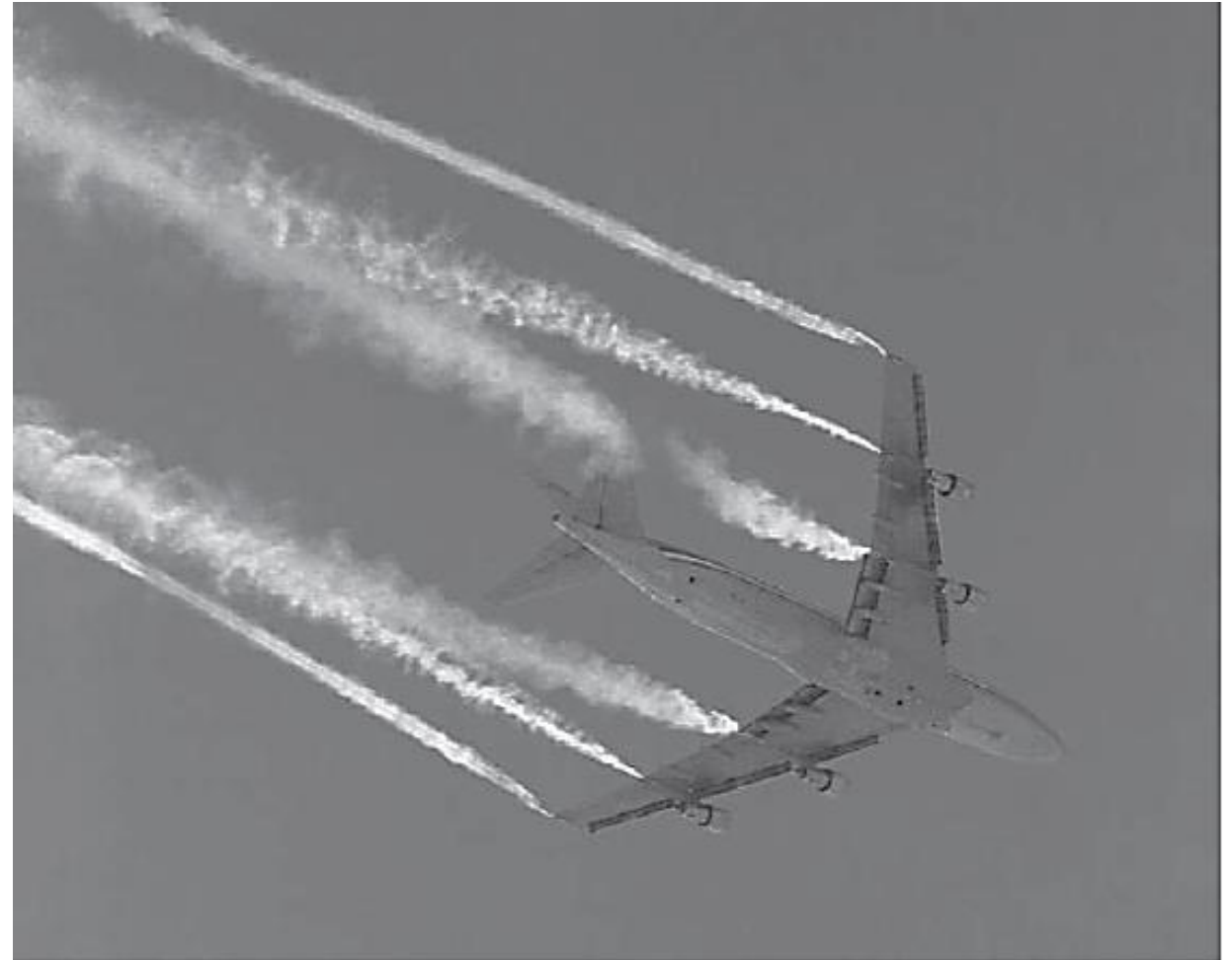
Figure 7.4 (Continued) (b) Streamwise vorticity shedding along the trailing edge of a Boeing 747 rolling up into wing-tip vortices (courtesy of NASA Dryden Flight Research Center).
