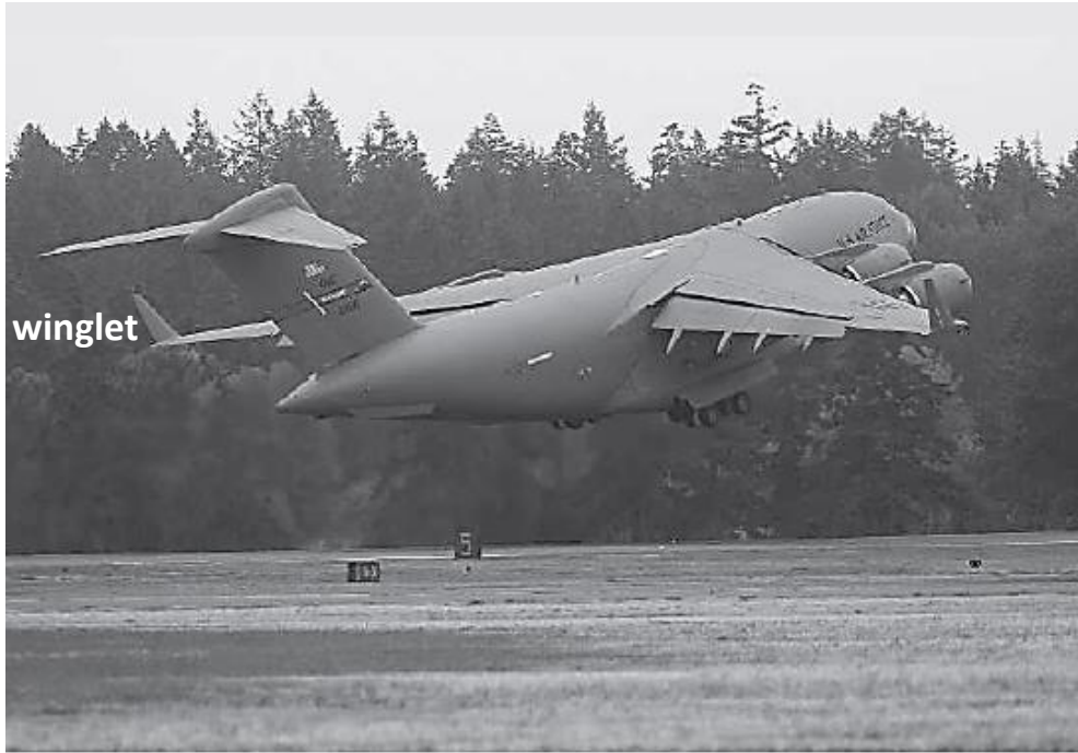
C-17 with wing flaps and leading-edge devices extended and winglets visible (U.S. Air Force photo by Abner Guzman)
